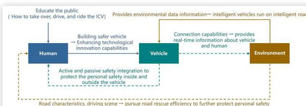
**FIGURE 9** Research and development(R&D) concepts, R&D architecture and R&D methods of vehicle safety for intelligent and connected vehicles
