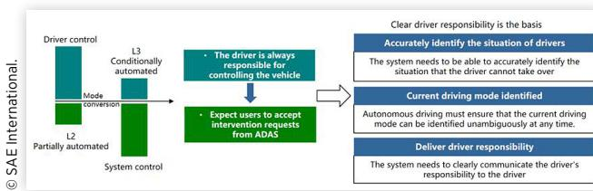
situation in which the driver and the system compete for control. Before the system makes a takeover request, the system needs to be able to accurately identify the situation that the driver cannot take over. If it is confirmed that the driver's status can take over the control of the vehicle, the system needs to clearly communicate the driver's responsibility to the driver, as shown in Fig 4.
