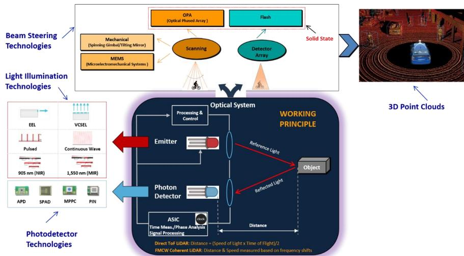
Figure 1. Working principle of LiDAR
