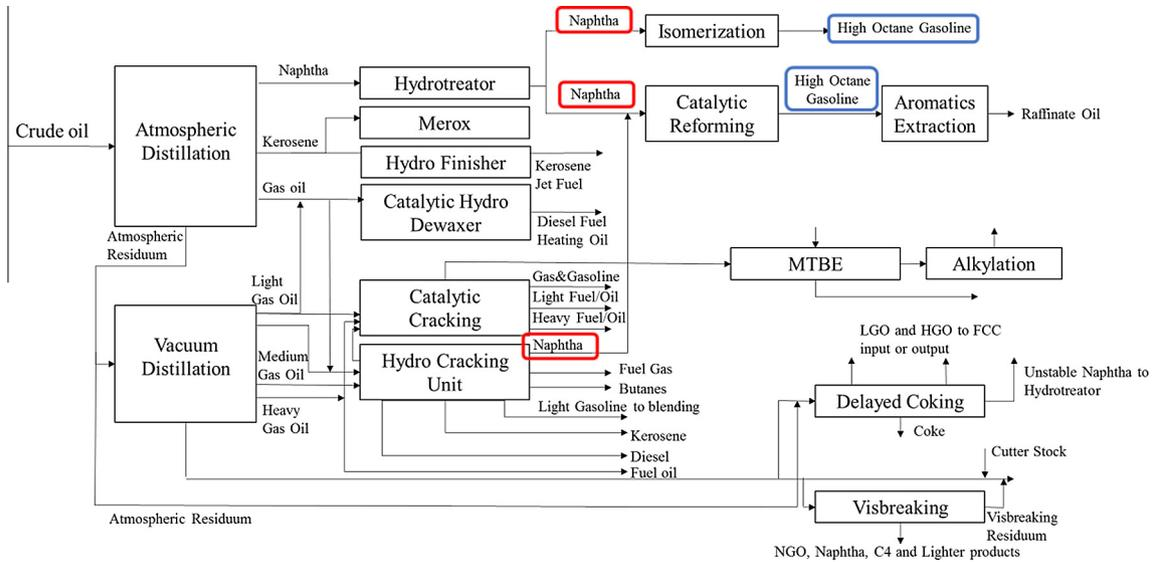
Fig. 1. Typical crude oil refining processes.
