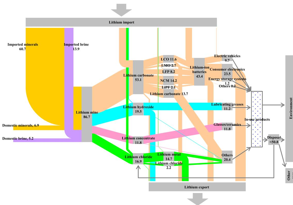
Fig. 5. Lithium flow in China for the year 2015.
