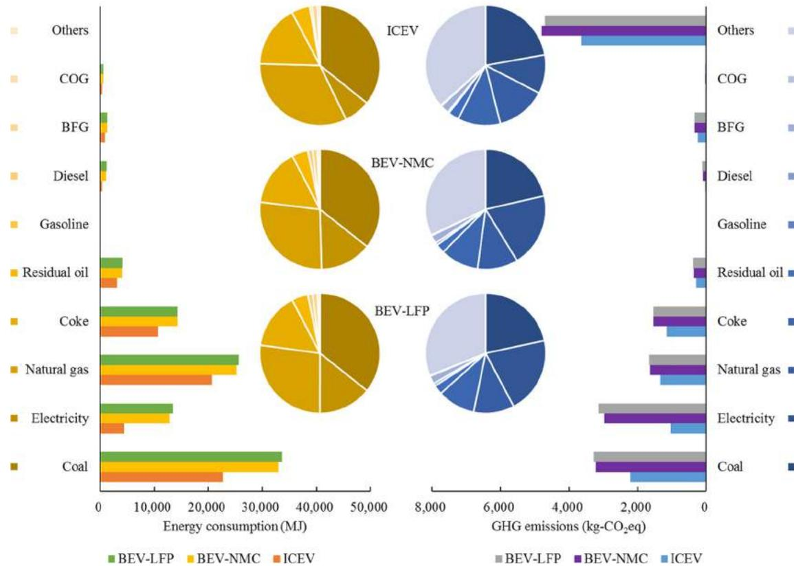
Fig. 5. Energy consumption and GHG emissions of each energy source.
