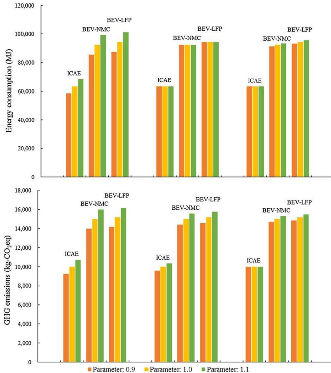
**Fig. 6.** Energy consumption and GHG emissions when (a) curb weight, (b) GHG emission factor of electricity production, (c) energy consumption and GHG emissions of Li-ion battery production are multiplied by sensitivity parameters.
