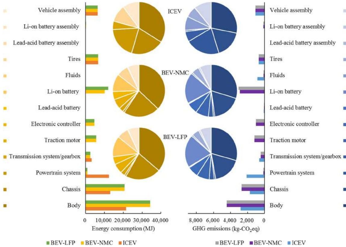
Fig. 3. Energy consumption and GHG emissions of each component.
