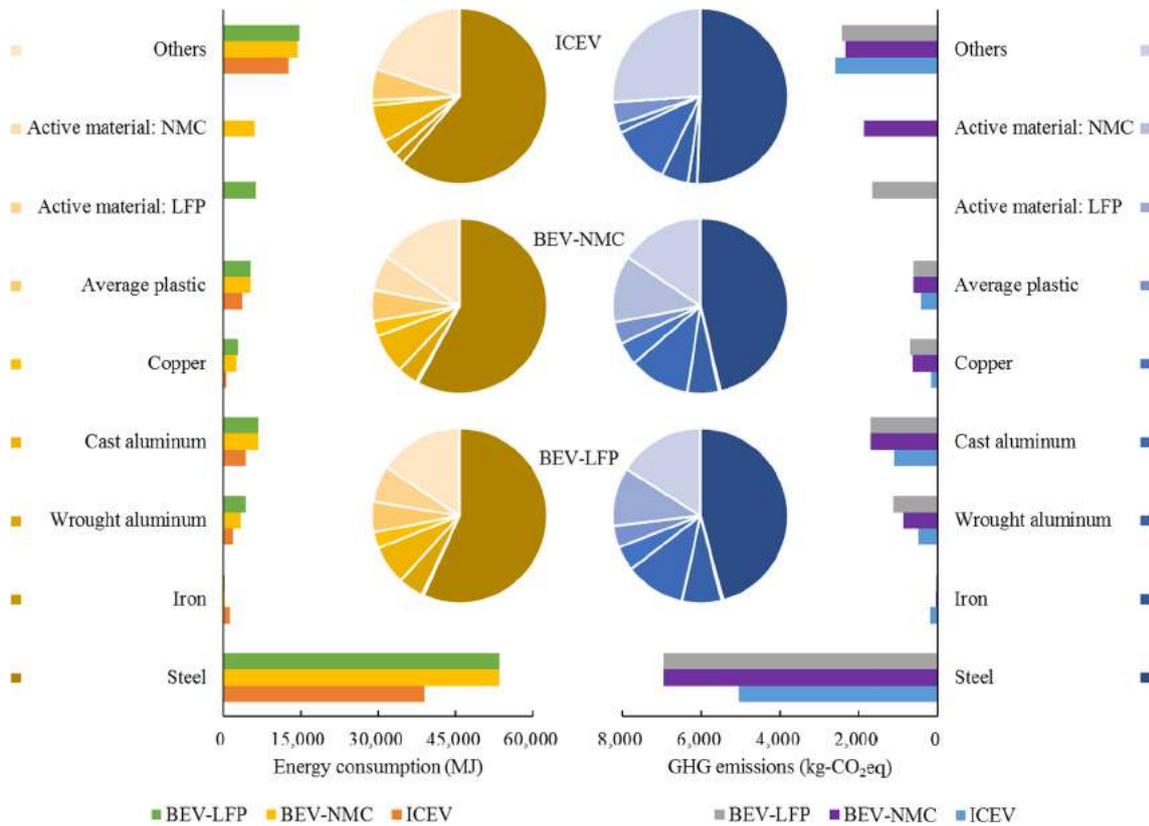
Fig. 4. Energy consumption and GHG emissions of each material.
