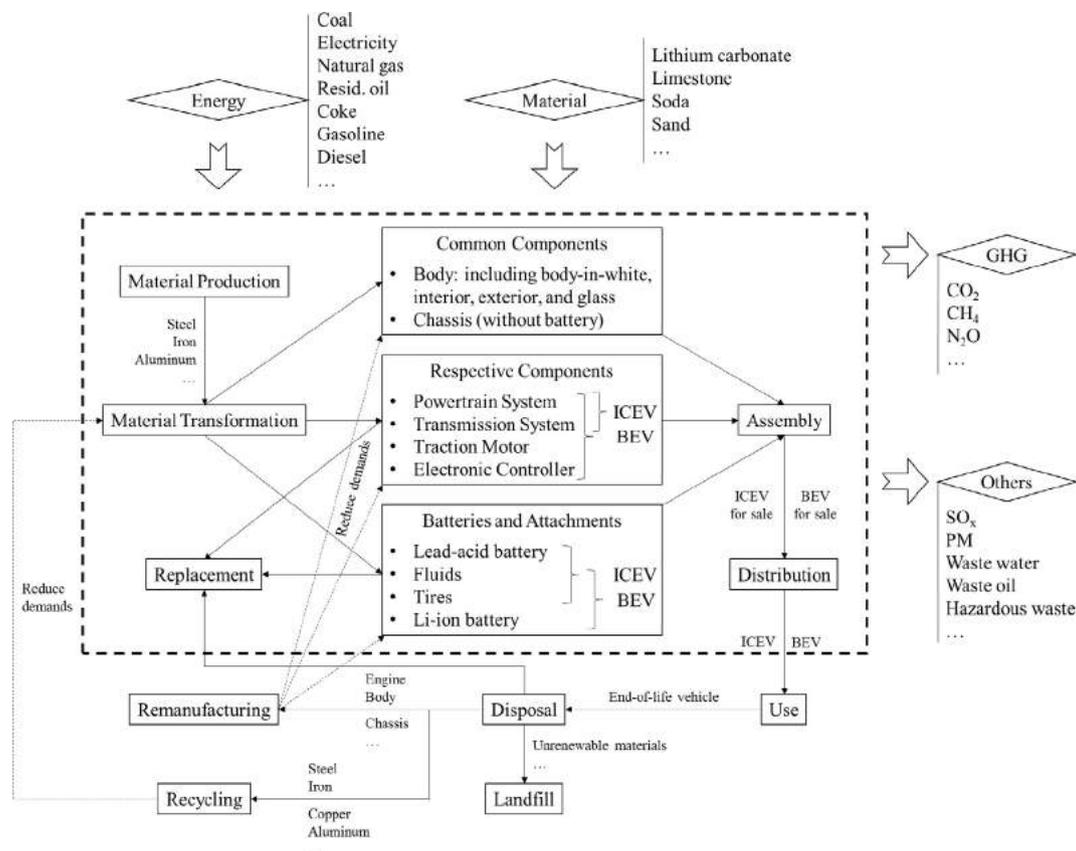
Fig. 1. Vehicle production model and boundary defined.
