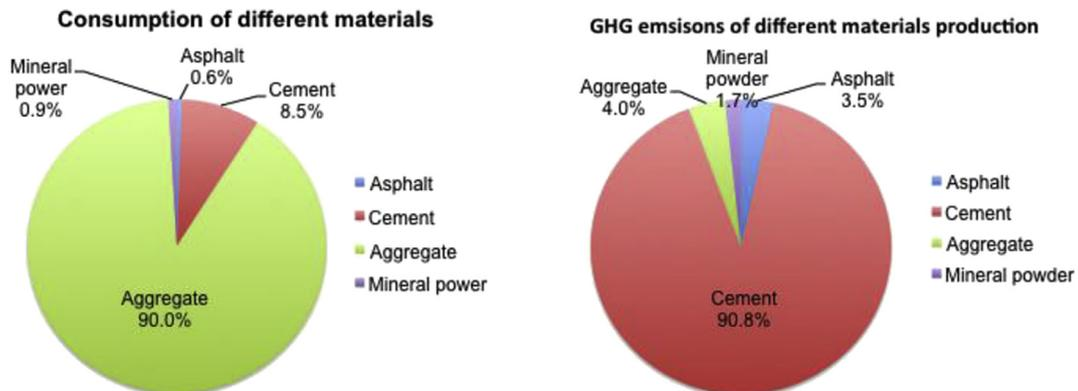
Fig. 8. Breakdowns of weight and GHG emissions by different materials.
