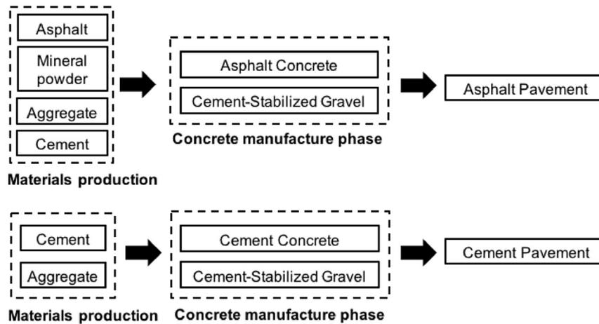
Fig. 3. System boundary for the calculation of GHG emissions from road construction.
