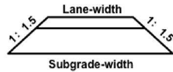
Fig. 5. The cross section of the road (Zhang and Liu, 2015).
