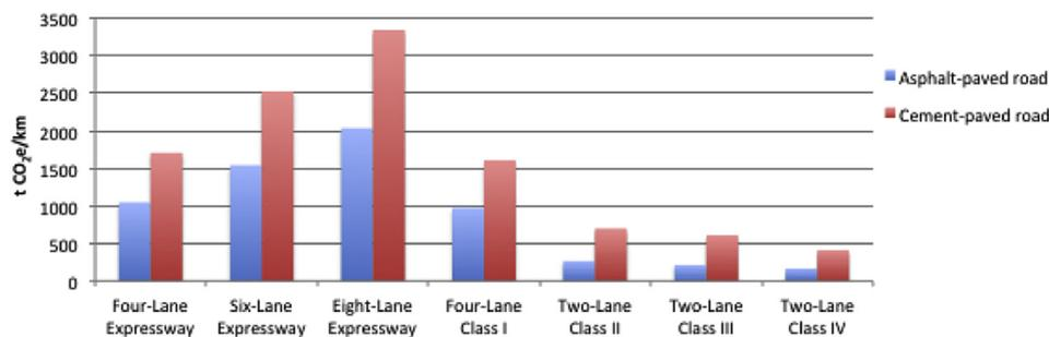
**Fig. 6.** GHG emissions intensities of different classes of roads.
