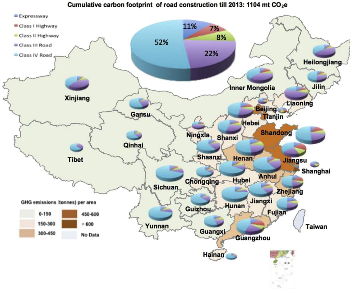
Fig. 7. The GHG emissions from road construction on the national and provincial levels.
