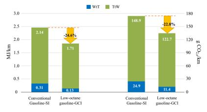
Fig. 3. Life cycle energy consumption and GHG emissions.
