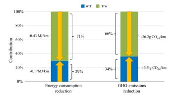
Fig. 4. The contributions of the WtT and TtW phases in reducing energy consumption and GHG emissions.
