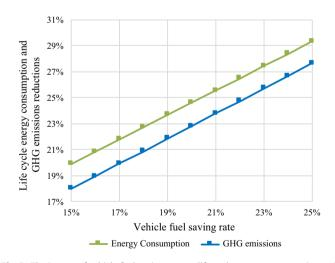
**Fig. 5.** The impact of vehicle fuel saving rate on life cycle energy consumption and GHG emissions reduction.
