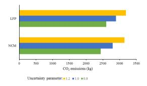
Fig. 3. Uncertainty of CO<sub>2</sub> emissions from battery production
