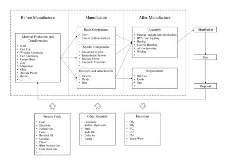
Fig. 1. Vehicle production system and boundary defined
