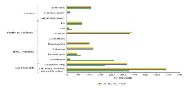
Fig. 2. Decomposition of CO2 emissions by different parts
